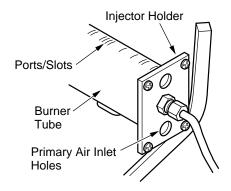
Figure 38 - Injector Holder On Outlet Burner Tube
